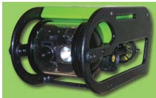
Figure 5-60 Photograph of the Remote Operating Vehicle used for collecting images from the removal and control sites at Maatsuyker Island, Tasmania. Model SeaBotix LBV300S2, www.seaviewsystems.com
